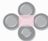
TS Cell Heat Radiation Space
