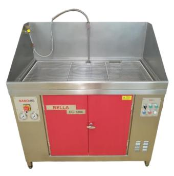
Ink tanks, application rollers, etc. are cleaned efficiently and sustainably with the HP specific Imaging Oil. The highlight is the integrated recycling system, which continuously removes ink particles from the Imaging Oil. This has the advantage that the dirty parts are always cleaned with a consistently clean Imaging Oil. This reduces operating costs and the volume of hazardous waste to a minimum.
